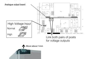
Gently move lug out a fraction with a screwdriver to release the backplate.
