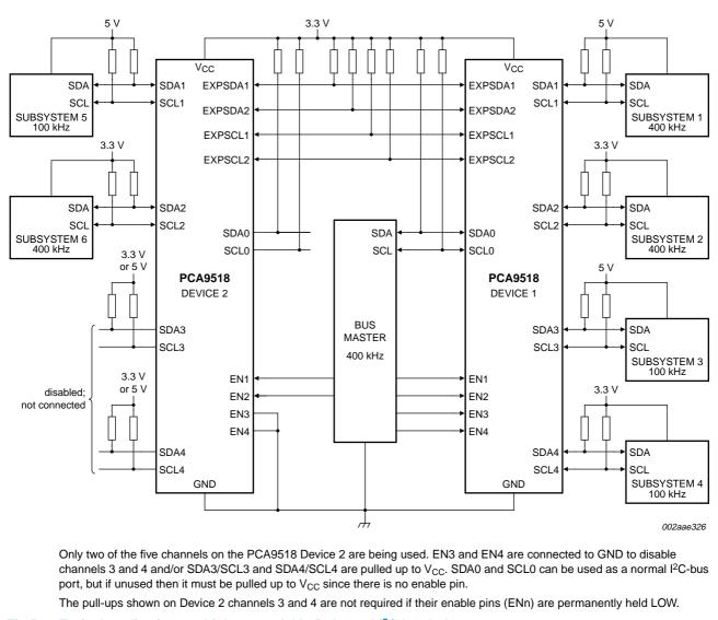
is 1  $\mu$ s or, when the bus 0 SDA reaches 0.7V<sub>CC</sub>, whichever occurs first. After both EXPSDA2 and EXPSDA1 are HIGH the rest of the SDA lines are allowed to rise. The same description applies for the EXPSCL1, EXPSCL2, and SCL pins.
