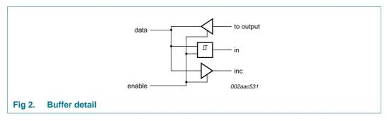
The output pull-down voltage of each internal buffer is set for approximately 0.5 V, while the input threshold of each internal buffer is set about 0.07 V lower, when the output is internally driven LOW. This prevents a lock-up condition from occurring.
