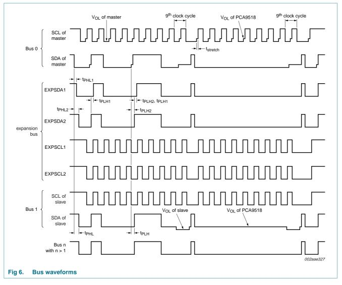
It is important to note that any arbitration or clock stretching events on Bus 1 require that the V<sub>OL</sub> of the devices on Bus 1 be 70 mV below the V<sub>OL</sub> of the PCA9518 (see V<sub>OL</sub>-V<sub>ILc</sub> in <u>Section 9 "Static characteristics"</u>) to be recognized by the PCA9518 and then transmitted to Bus 0.
