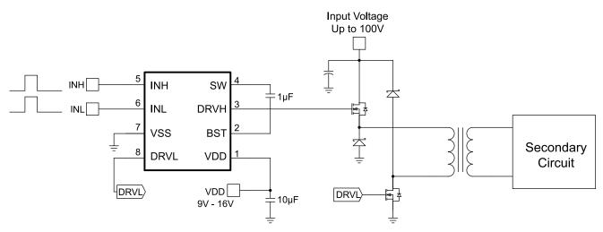
Figure 5—Two-Switch Forward Converter
