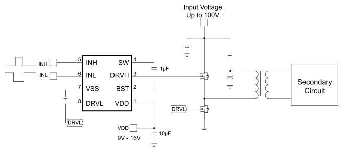
Figure 4—Half Bridge Converter
