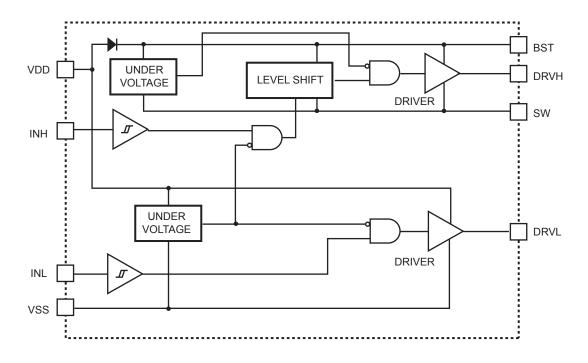
Figure 2—Function Block Diagram
