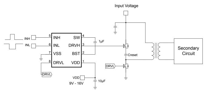
Figure 6—Active-Clamp Forward Converter
