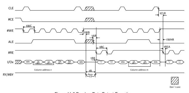
Figure 11-9 Random Data Output Operation
