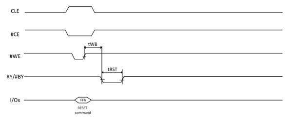
Figure 9-17 Reset Operation
