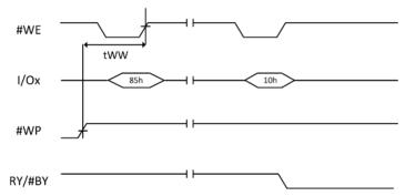
Figure 9-27 Program for Copy Back Enable
