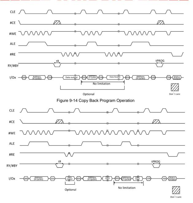
Figure 9-15 Copy Back Operation with Random Data Input
