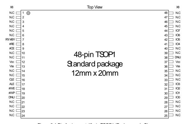
Figure 3-1 Pin Assignment 48-pin TSOP1 (Package code S)
