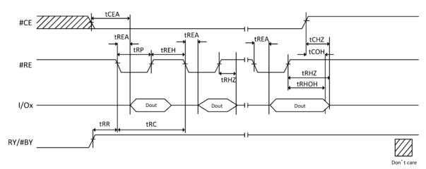
Figure 11-4 Serial Access Cycle after Read
