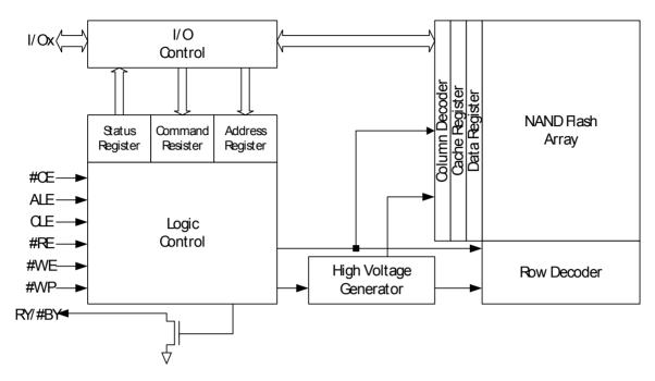
Figure 5-1 NAND Flash Memory Block Diagram
