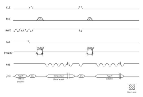
Figure 9-4 Last Address Cache Read Operation
