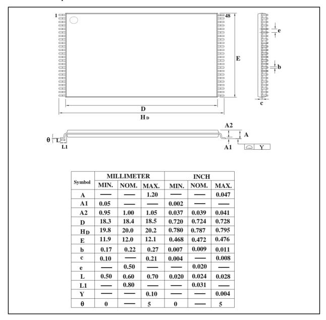
Figure 13-1 TSOP 48-PIN 12X20mm
