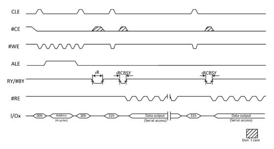
Figure 9-2 Sequential Cache Read Operations
