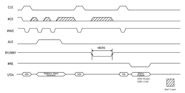
Figure 9-16 Block Erase Operation
