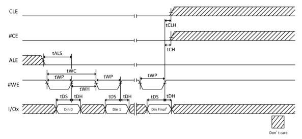
Figure 11-3 Data Latch Cycle
