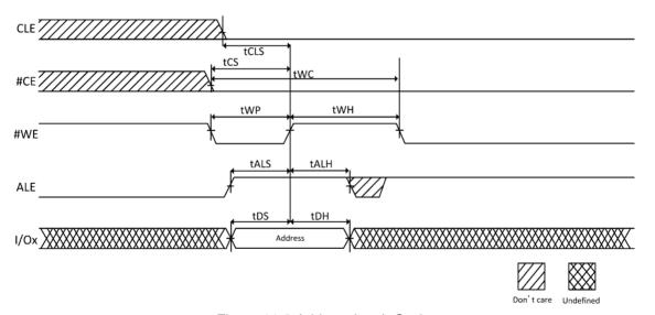
Figure 11-2 Address Latch Cycle
