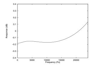
Figure 34 De-Emphasis Frequency Response (48kHz)
