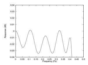
Figure 22 DAC Digital Filter Frequency Response-Type 0
