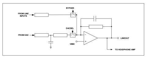
Figure 8 Line Output Schematic
