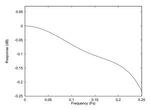
Figure 28 DAC Digital Filter Frequency Response-Type 3
