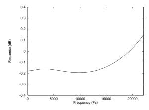
Figure 32 De-Emphasis Frequency Response (44.1kHz)
