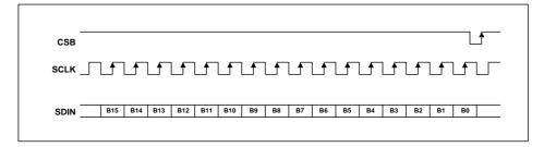
Figure 20 3-Wire Serial Interface
