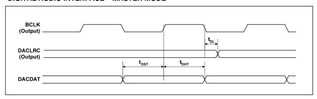
Figure 2 Digital Audio Data Timing - Master Mode
