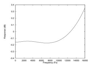
Figure 30 De-Emphasis Frequency Response (32kHz)
