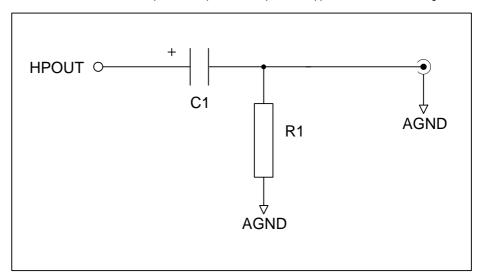
Figure 11 Headphone Output Application Drawing
