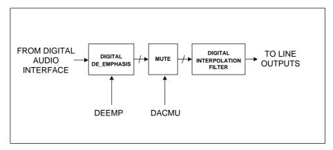
Figure 6 DAC Filter Schematic
