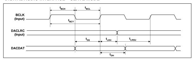
Figure 3 Digital Audio Data Timing - Slave Mode
