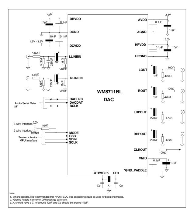
Figure 36 External Components Diagram
