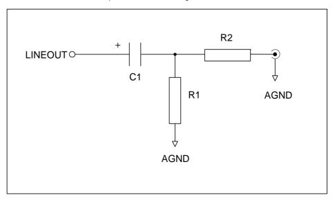
Figure 9 Line Outputs Application Drawing
