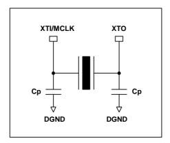
Figure 12 Crystal Oscillator Application Circuit
