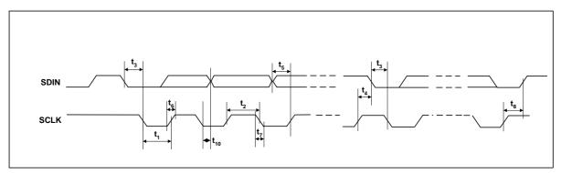
Figure 5 Program Register Input Timing – 2-Wire MPU Interface Timing
