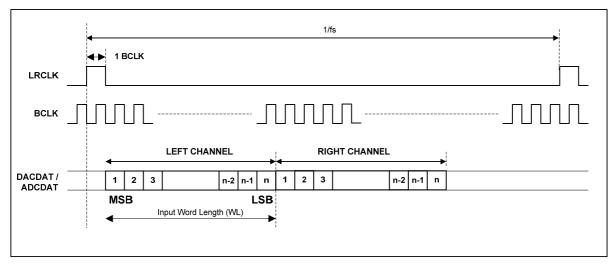
Figure 16 DSP/PCM Mode Audio Interface (mode A, LRP=1)
