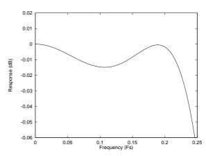
Figure 26 DAC Digital Filter Frequency Response-Type 2
