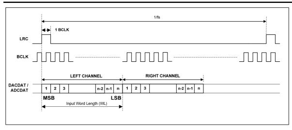
Figure 17 DSP/PCM Mode Audio Interface (mode B, LRP=0)
