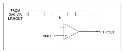
Figure 10 Headphone Amplifier Schematic
