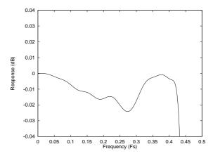
Figure 24 DAC Digital Filter Frequency Response-Type 1
