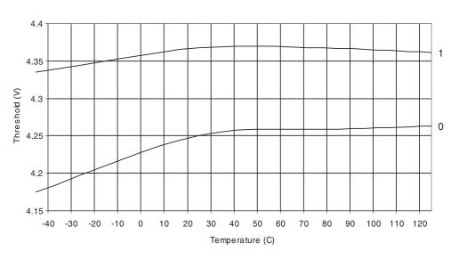
Figure 23-30. BOD Threshold vs, Temperature (BODLEVEL is 2.7V)
