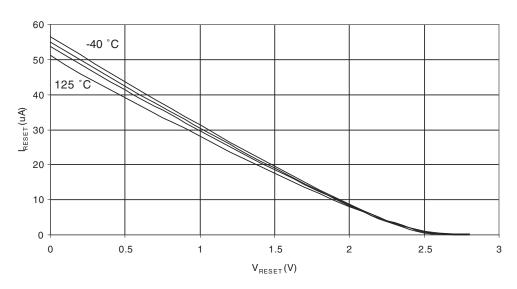
Figure 23-18. Reset Pull-up Resistor Current vs. Reset Pin Voltage (V<sub>CC</sub> = 5V)
