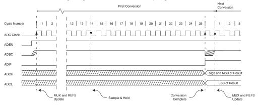
Figure 18-5. ADC Timing Diagram, Single Conversion
