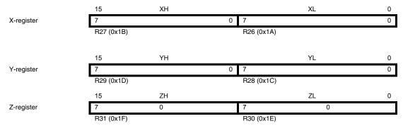
In the different addressing modes, these address registers have functions as fixed displacement, automatic increment, and automatic decrement (see the instruction set summary for details).
