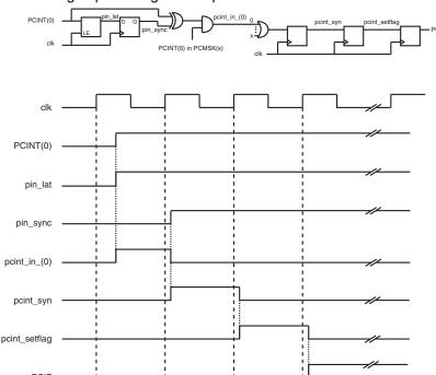
Figure 11-1. Timing of pin change interrupts
