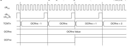
Figure 13-11 on page 83 shows the setting of OCF0A and the clearing of TCNT0 in CTC mode and fast PWM mode where OCR0A is TOP.
