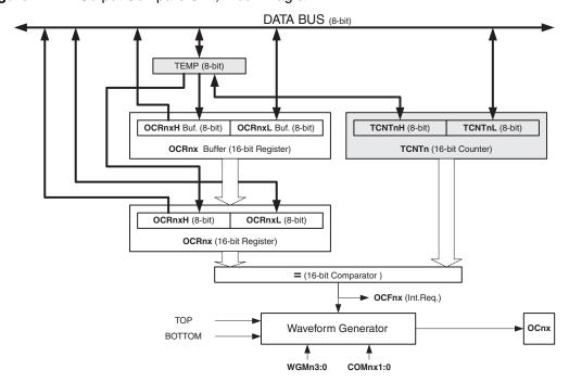
Figure 14-4. Output Compare Unit, Block Diagram
