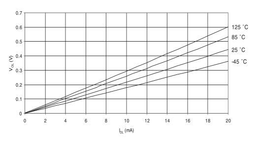
Figure 23-21. I/O Pin Output Voltage vs. Source Current (V<sub>CC</sub> = 3V)
