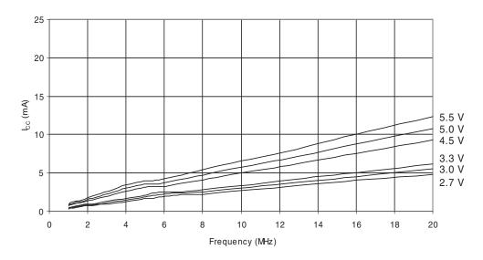
Figure 23-4. Active Supply Current vs. frequency (1 - 20MHz) - Temp.=125°C
