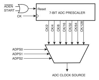
By default, the successive approximation circuitry requires an input clock frequency between 50kHz and 200kHz to get maximum resolution. If a lower resolution than 10 bits is needed, the input clock frequency to the ADC can be higher than 200kHz to get a higher sample rate. The ADC module contains a prescaler, which generates an acceptable ADC clock frequency from any CPU frequency above 100kHz.
