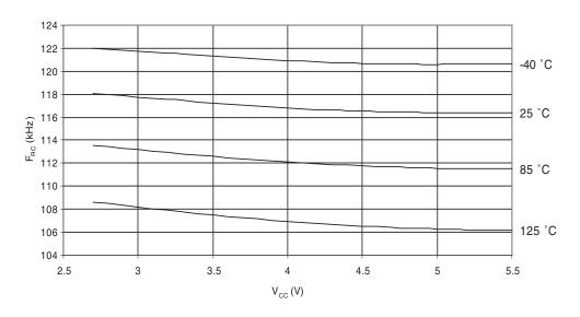
Figure 23-33. Calibrated 8MHz RC Oscillator Frequency vs.  $V_{\rm CC}$
