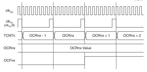
Figure 14-12 on page 112 shows the count sequence close to TOP in various modes. When using phase and frequency correct PWM mode the OCR1x Register is updated at BOTTOM. The timing diagrams will be the same, but TOP should be replaced by BOTTOM, TOP-1 by BOTTOM+1 and so on. The same renaming applies for modes that set the TOV1 flag at BOTTOM.
