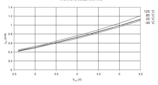
Figure 23-7. Active Supply Current vs. V<sub>CC</sub> (Internal RC Oscillator, 128kHz)
