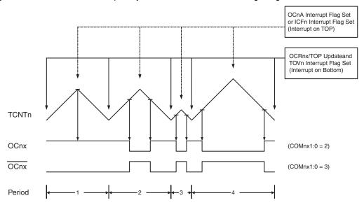
The timer/counter overflow flag (TOV1) is set on the same timer clock cycle on which the OCR1x registers are updated with the double buffer value (at bottom). When either OCR1A or ICR1 is used for defining the top value, the OC1A or ICF1 flag is set accordingly when TCNT1 has reached top. The interrupt flags can then be used to generate an interrupt each time the counter reaches the top or bottom value.
