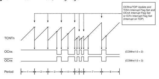
The timer/counter overflow flag (TOV1) is set each time the counter reaches top. In addition, the OC1A or ICF1 flag is set on the same timer clock cycle on which TOV1 is set when either OCR1A or ICR1 is used for defining the top value. If one of the interrupts are enabled, the interrupt handler routine can be used for updating the top and compare values.
