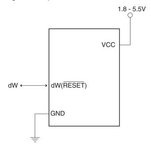
Figure 19-1 on page 156 shows the schematic of a target MCU, with debugWIRE enabled, and the emulator connector. The system clock is not affected by debugWIRE and will always be the clock source selected by the CKSEL Fuses.
