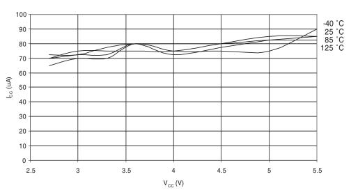
Figure 23-39. Programming Current vs. V<sub>CC</sub>
