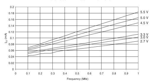
**Figure 23-42.** Reset Supply Current vs.  $V_{CC}$  (1 - 20MHz, Excluding Current Through the Reset Pull-up)
