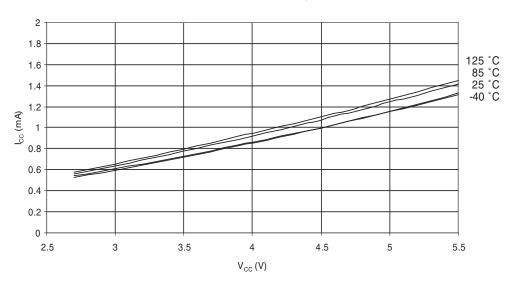
Figure 23-11. Idle Supply Current vs.  $V_{CC}$  (Internal RC Oscillator, 1MHz)
