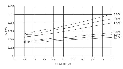
Figure 23-9. Idle Supply Current vs. Frequency (1 - 20MHz)
