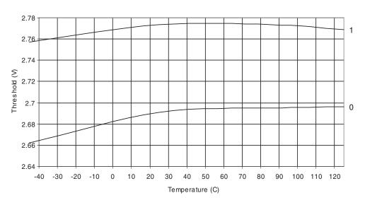
Figure 23-31. BOD Threshold vs. Temperature (BODLEVEL is 1.8V)
