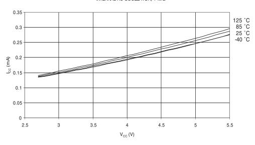
Figure 23-12. Idle Supply Current vs.  $V_{CC}$  (Internal RC Oscillator, 8MHz)
