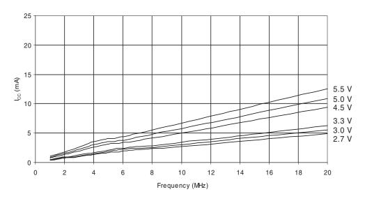
$\textbf{Figure 23-5.} \quad \text{Active Supply Current vs. } V_{\text{CC}} \text{ (Internal RC Oscillator, 8MHz)}$
