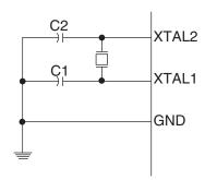
The Oscillator can operate in three different modes, each optimized for a specific frequency range. The operating mode is selected by the fuses CKSEL3..1 as shown in Table 7-3 on page 27.
