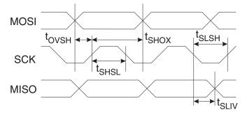
Figure 22-4. Serial Programming Waveforms
