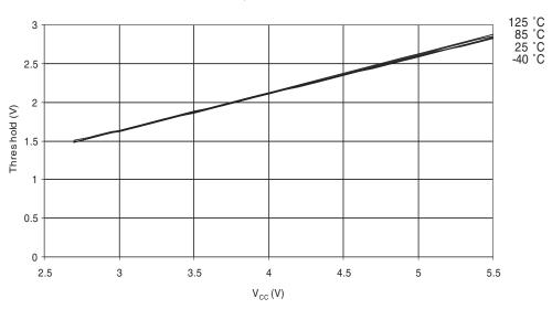
Figure 23-27. Reset Input Threshold Voltage vs.  $V_{CC}$  ( $V_{IL}$ , IO pin Read as '0')
