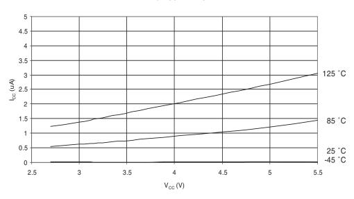
Figure 23-14. Power-down Supply Current vs. V<sub>CC</sub> (Watchdog Timer Enabled)
