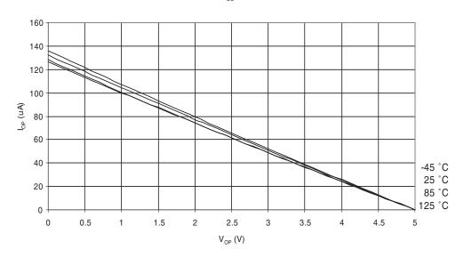
Figure 23-17. Reset Pull-up Resistor Current vs. Reset Pin Voltage (V<sub>CC</sub> = 2.7V)
