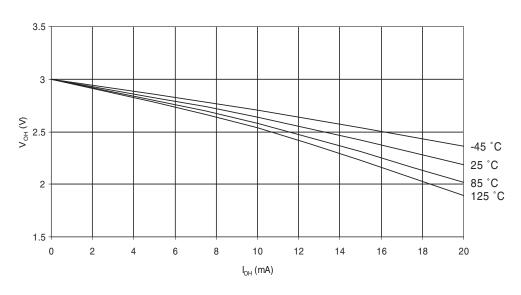
Figure 23-22. I/O Pin output Voltage vs. Source Current ( $V_{CC} = 5V$ )
