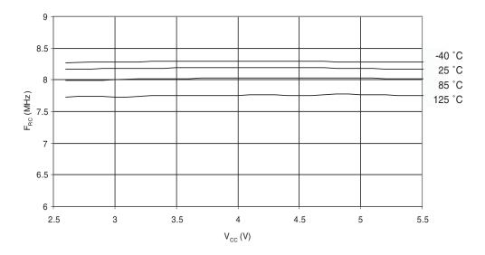
Figure 23-34. Calibrated 8MHz RC oscillator Frequency vs. Temperature
