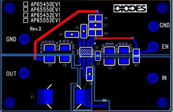
Figure 7: PC Board Layout for SO-8EP
