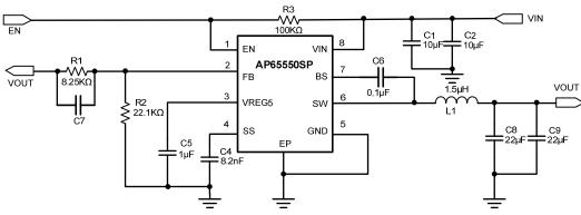
Figure 3. Typical Application of AP65550SP (SO-8EP) Evaluation Board
