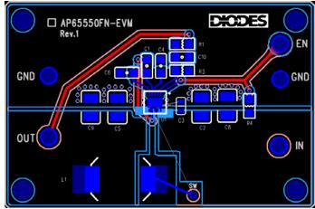
Figure 8: PC Board Layout for U-DFN3030-10
