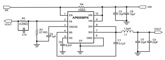
Figure 4. Typical Application of AP65550FN (U-DFN3030-10) Evaluation Board
