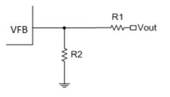
Figure 6. Feedback Divider Network
