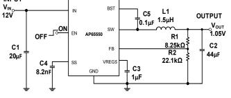
Figure 1. Typical Application Circuit
