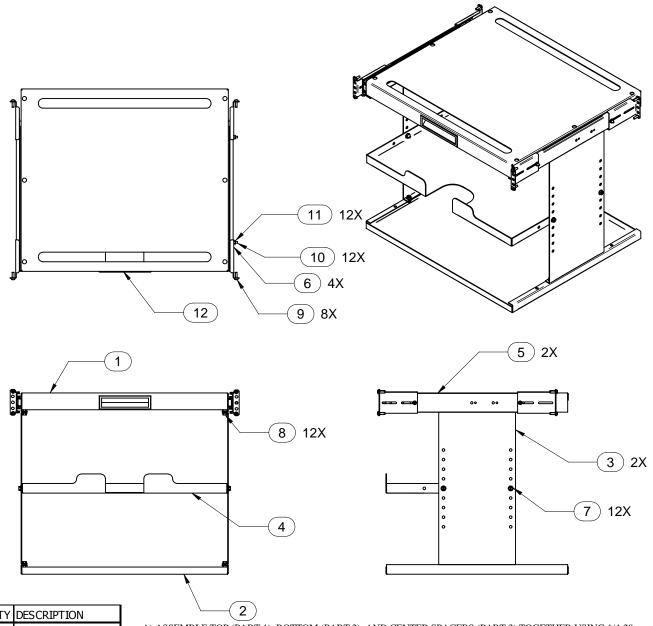
PART # QTY TOP 2 BOTTOM 3 2 CENTER SPACER 4 PAPER SHELF BALL BEARING SLIDE 6 SLIDE BRACKET 1/4-20 CAP SCREW 12 8 1/4-20 KEP NUT 9 10-32 SCREW 10 12 8-32 SCREW 11 8-32 KEP NUT SOUTHCO PULL 12
